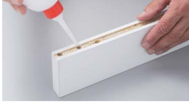
1. Pour a few drops of glue in the holes of posts
