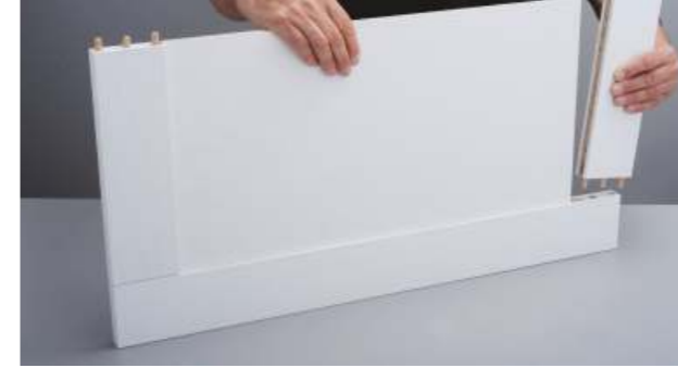
5. Insert the second side beam with a lateral post
