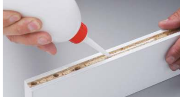
2. Put a line of glue along the entire groove on lateral posts and side beams
