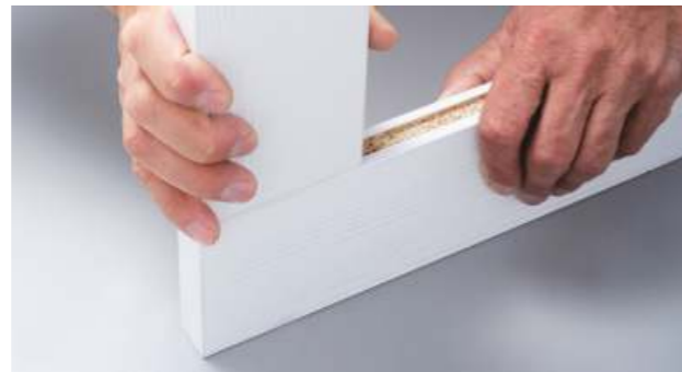
2. Put a line of glue along the entire groove on lateral posts and side beams
