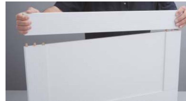
6. Close the frame with the remaining post
